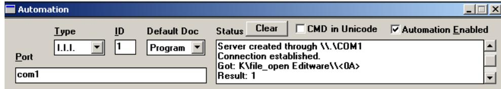
When you have successfully communicated with the Deko, the automation box will show that it received the command from the Fastrack.
