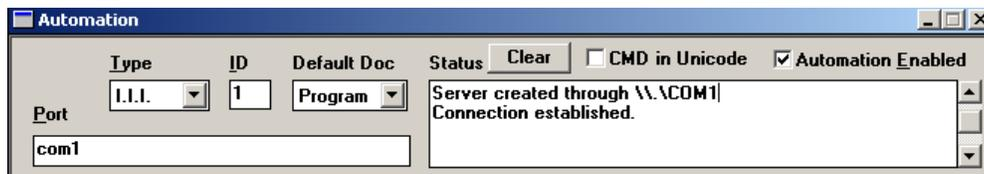
Once you click on **Automation Enabled**, you will see that it says **Connection established**. However, this only means that it is talking with its COM port and not necessarily with the Fastrack. It is still possible to have a wiring problem or an incorrect setting on the Fastrack and still get the “Connection established” prompt.
